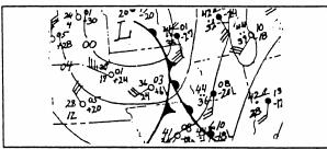
Variations in altimeter settings between weather reporting points is caused by unequal heating of the earth's surface.
